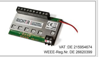
The RICHTER PPX Piezo Preamp is a unique circuit featuring dedicated channels for each string of your bass or guitar. It is combinable with the piezo upgrade for ETS bridges.
