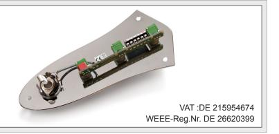
The RICHTER JB PASSIVE control plate is an easy mounting component for passive bass guitars like the Jazz Bass TM. It provides two independent volume pots and one tone control pot. A shielded PCB replace the wiring - therefore no shielding inside the instrument is required.
